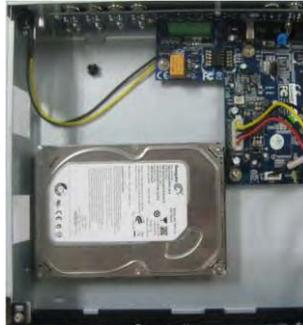
Fig 2-1 Connect HDD
