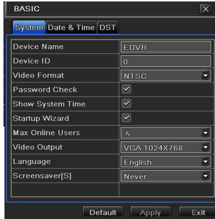
Fig 4-3 basic configuration-basic
